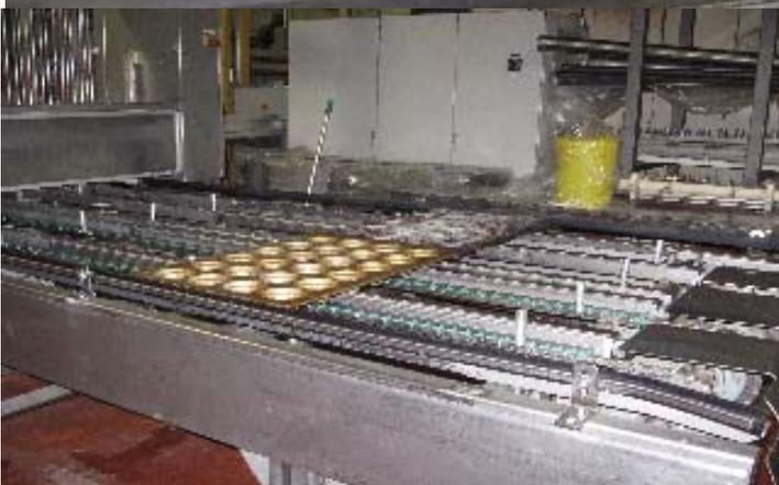
Automated oven chain lubrication system in a production bakery. Project included system design, supply and installation of lubricant application equipment, control system to cycle and monitor system operation.
