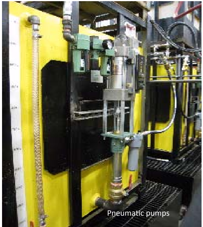
Portable tote tanks located on permanent lower tank and containment system with level controls and low level pump shut protection..
