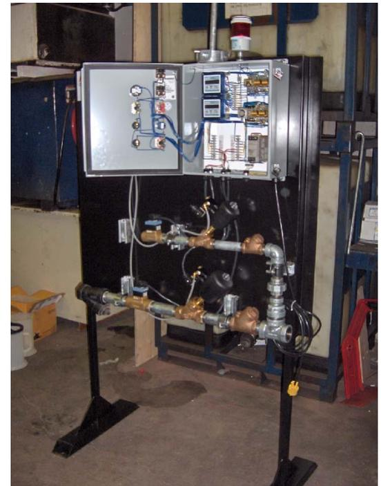
Pro/Mark model PVF-7A Processor controlled proportioning system provides accurate and consistent proportioning of heavy stamping fluids. Up to 7 selectable pre-set ratios and full system shut down if there is no water or no concentrate. Optional blending tank with agitator available.
