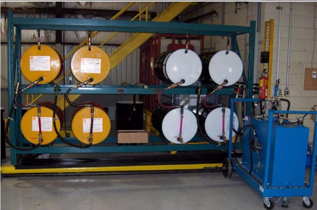
Truck assembly plant wanted to use portable lube carts to take fluids to the production line. The carts are equipped with Pro/Mark's unique self-fill kit which eliminates the need for separate transfer pumps to fill the cart reservoirs. The carts are filled by coupling to racked drums and stationary bulk tanks. Cards are modular in design to accommodate reservoir changes.
