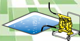
PUMP INSTALLED ON A MOBILE UNIT
