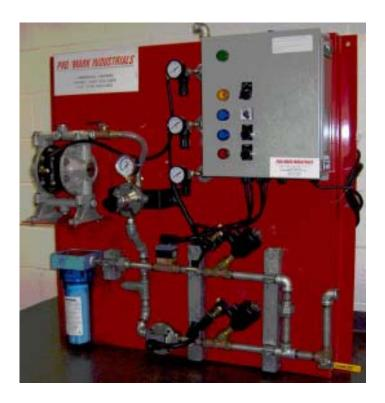
Pro/Mark's PVF Series proportioners are designed to provide precise, consistent blending of two component fluids.
