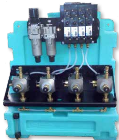
Four PresSpray Units on a Four Gallon Reservoir Each PresSpray dispenses fluid when the solenoid that controls it is actuated. An LSP Controller controls when these solenoids actuate.
